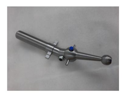
Use plenty of grease around the ball of the lower pivot and in the top of the turret where the pivot sits. Insert the pressure spring and nylon pad into the hole in the lower pivot. Pushing the pressure spring in drop the pivot into the turret. Secure the pivot into the turret with the washer and M6 bolt.
