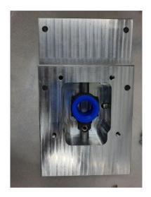
The main gearstick turret will need slight modification. You will notice the M6 adjustment bolts for the bias spring are different heights. The taller one will need filing or grinding down to the same height as the other. This is to allow enough adjustment on the spring as the turret has been turned around. The marker pen shows the areas that need to be removed.
