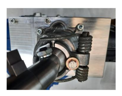
Fit the 2 dowels into the top of the gearbox. Take your time don't drop them. Use RTV around the top/ mating face of gearbox. Drop the main billet assembly onto the top of the gearbox. Ensure that the 2 selectors slide together. You may need to use a soft mallet just to pop the assembly onto the dowels. Use 2x M8 and 2x M8 fixings and washers.
