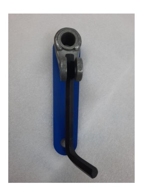
Get the part setup so that it is held in the correct place and flat to the shoulder on the part. Weld around the part and the plate just like the weld that you cut off to remove the old plate. Do not weld the inside. Only around the front. Once welded file or grind the weld flat and smooth so that the bush pushes back in. Repaint.
