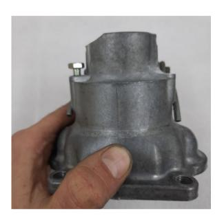
On the turret there is a washer that bolts down to hold the lower pivot into the turret. The top, left hand side, edge of the turret needs to be filed or ground down to the same height. You can go all the way around if you wish to make the top all the same height.
