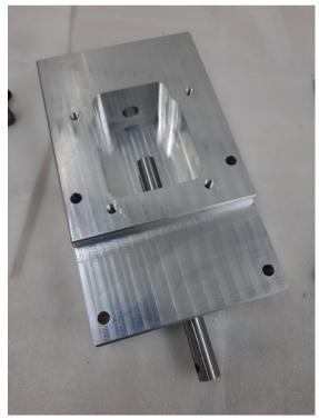
Turn the main billet over and slide the gearbox selector onto the end of the shaft in the underside pocket. Using a punch and hammer knock the roll pin through the gearbox selector and selector shaft.
