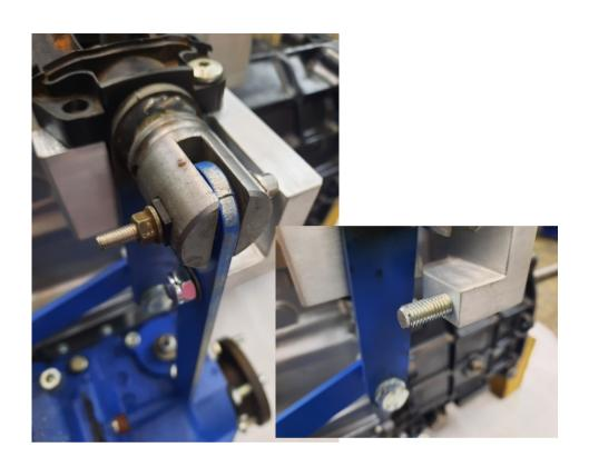
Drop a washer onto the top of both the M6 fixings then the second Difflock linkage plate.
