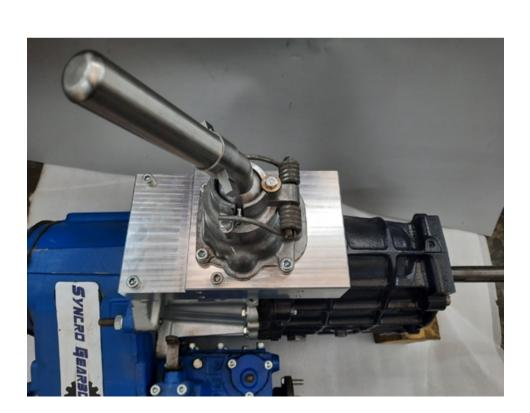
Put the Puma gearstick lever onto the top pivot. Make sure all the gears select. Put it into third. Adjust the M6 bolts until they touch the bias spring. Take it out of gear and make sure that third and fourth gear are in a straight line. With the bias spring set correctly third gear should be straight forward from its neutral position. Tighten the locking nuts on the adjustment bolts to set.
