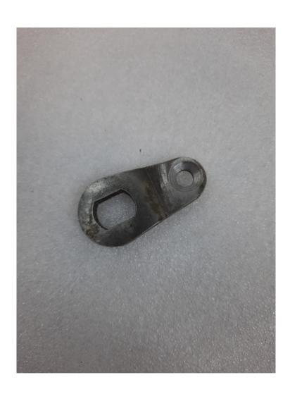
The Puma Difflock lever needs modification to work with the kit. Pull main Difflock/ High-low gearstick off the top. They are tight. Will need a lot of force. Using a screwdriver, pull the clips open on one side to pop the plastic housings off the mechanism. Use a punch and hammer to knock the roll pin out of the Difflock part on the end to remove.
