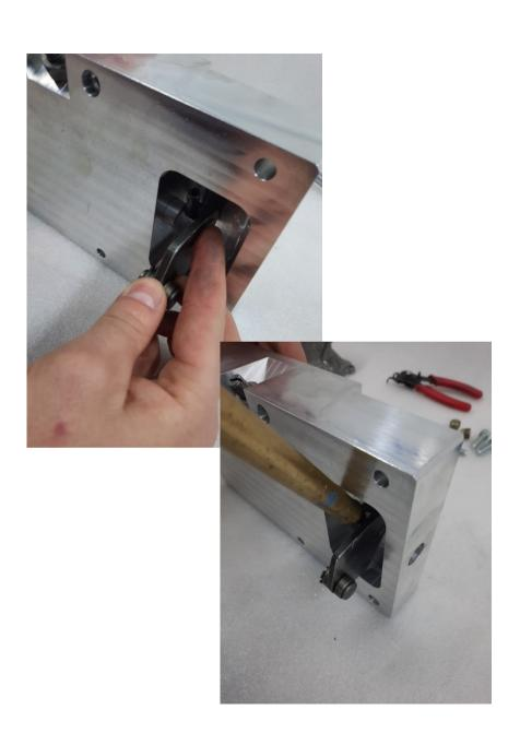
Turn the main billet back over the right way up. Line the yoke up with the hole in the selector shaft. Using Loctite, put the grub screw into the yoke and into the selector shaft. Inset the M18 plug into the end of the selector shaft hole to blank off.
