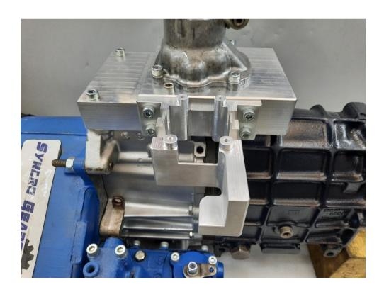
Take the High-low selector off the top of the transfer box. Put an M10 fixing through the hole in the selector, with washer and bolt up tight. Make sure the bolt goes through from the gearbox side. Make sure that the bolt is straight and parallel to the top of the selector housing. After many years of abused the swan shaped selector may be bend. Use a vise to straighten. Put the selector back on the transfer box using RTV.
