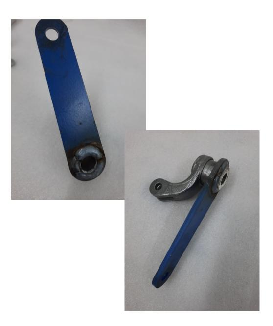
The lever can now be reassembled. First check that the modified part fits and turns smoothly in the bottom housing. Put the lever mechanism back together just as it came apart. Use the new clevis pin and clip provided in the kit to replace the rivet drilled out. Pop the Difflock part back on the end with the roll pin. Use plenty of grease around all of it and around where the assembly sits in the plastic housings.
