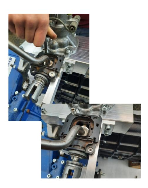
Fit the 2, 3d printed bushes to the top of the Difflock linkage with M5 fixing. Don't bolt to tight. Make sure they are free to move. Put an M6x40mm countersunk fixing in from the underside with washer and bolt up tight.
