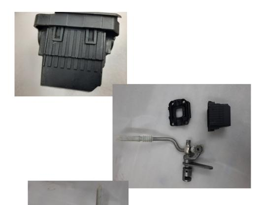
You will see the assembly is riveted together. Use a drill to take the top of the rivet and knock the rivet out with a punch and hammer. The assembly will now come apart.
