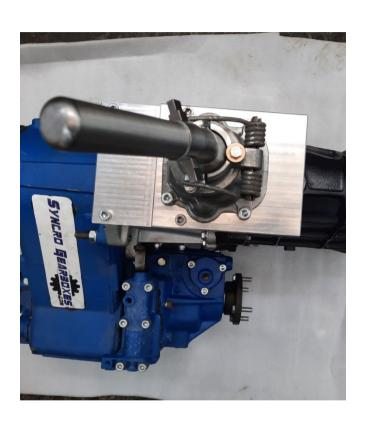
Using a screwdriver or Allen key push the bias spring over the pegs in the lower pivot. Take care as the spring is strong. Do one side at a time.
