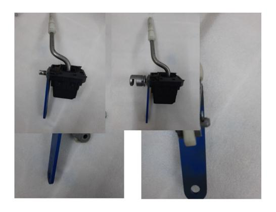
The lever can be pushed into the billet. It is a tight fit. Use the original M5 shoulder bolts to secure it into the billet.
