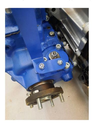
to the one in the transfer box selector. Leave loose for now. Put the new High-low linkage plate onto the 2 bolts. Work out how many washers you need on the transfer box end to evenly spacer the linkage so that's its straight. Once worked out. Fit the washers, do the bolt in the lever end up tight. Then fit 2 nyloc nuts just up snug. Operate the High-low and make sure that it selects nicely.
