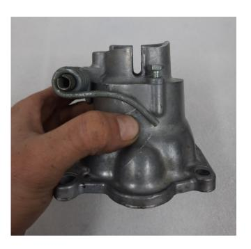
Ensure the selector shaft is nice and smooth before going any further and has plenty of lubrication. Fill the bush with grease. Use RTV around the bottom/ mating face of the turret to seal it to the main billet. Once the modifications have been made to the turret it can be bolted to the main billet with 4x M8x25mm fixings and washers.
