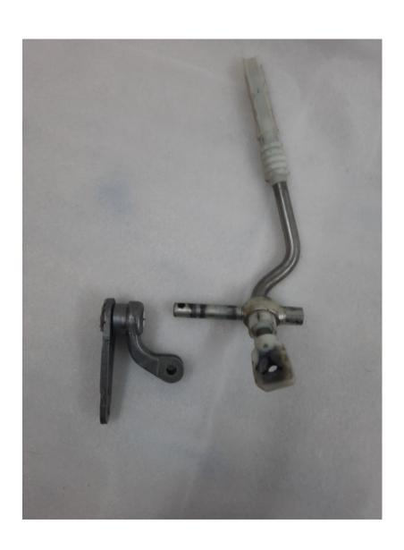
Once you have the part separated from the assembly shown on the adjacent page pop the bush out. Carefully trim around the weld with a hacksaw or grinder to remove the plate. Please take you time not to cut too much and scrap the part. The plate should just pop off once you have cut all the weld.
