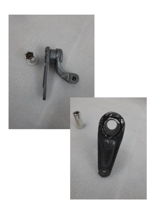
File around the edge of the part so that it is round and has a clean edge. Use the new plate provided in the kit, file until it fits flat to the shoulder on the part. The plate needs to be aligned to the part to ensure the lever is in the correct place.
